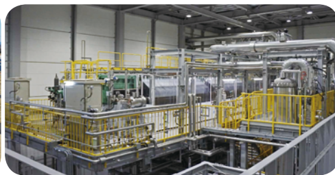
[10MW-class large-scale alkaline water electrolysis system]
